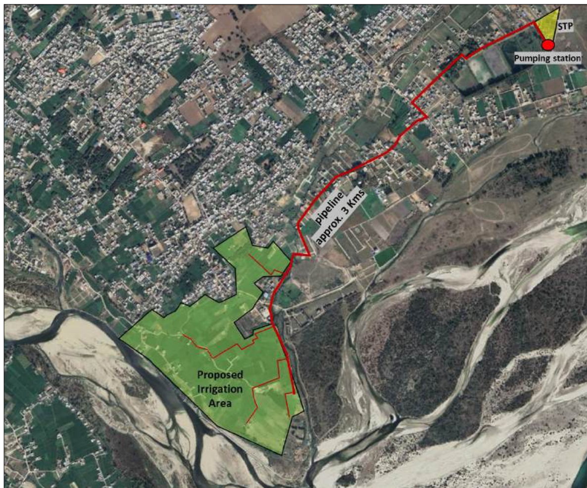
Image 7-35: Proposed Pipeline for reuse of treated used water
