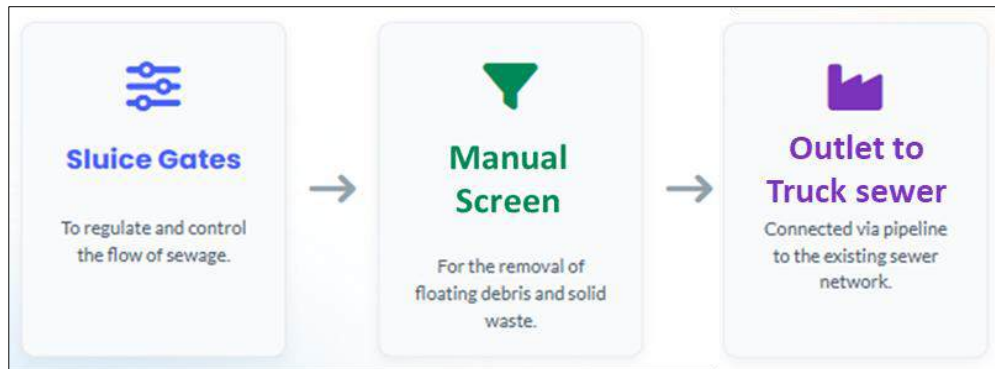
Image 7-6: Flow arrangement of proposed I &D Structure
